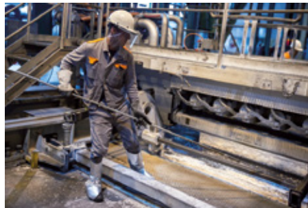
The thinly rolled steel strips are introduced into the galvanizing system. A protective gas mixture of nitrogen and hydrogen ensures that the material does not react with the oxygen before it is dipped into the 450 degrees hot zinc bath. The hydrogen for this is to come from the "Salzgitter Clean Hydrogen" project in future.
