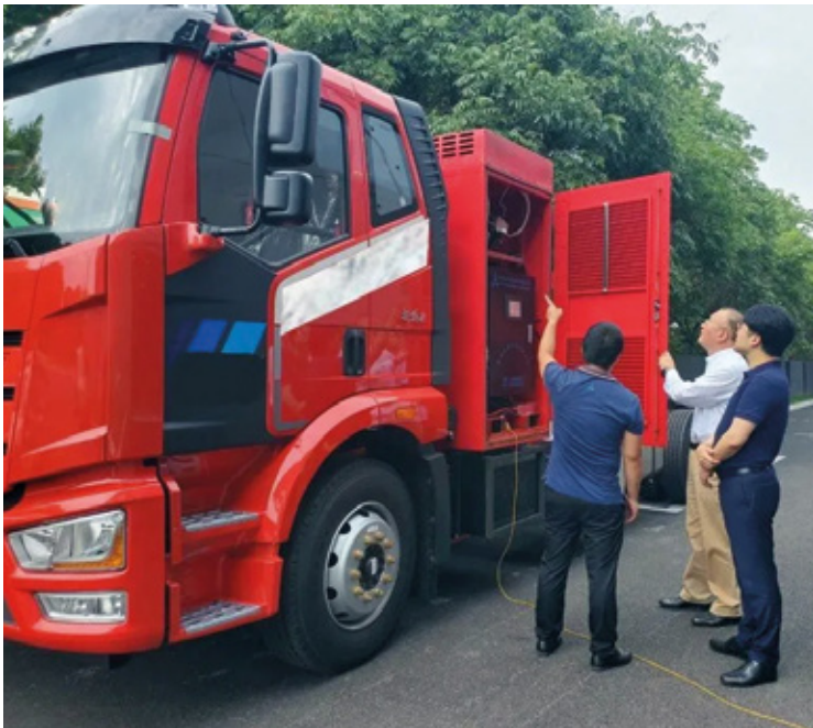
M-Series hydrogen generator (pictured above) has been incorporated onto a medium-duty fuel cell truck
