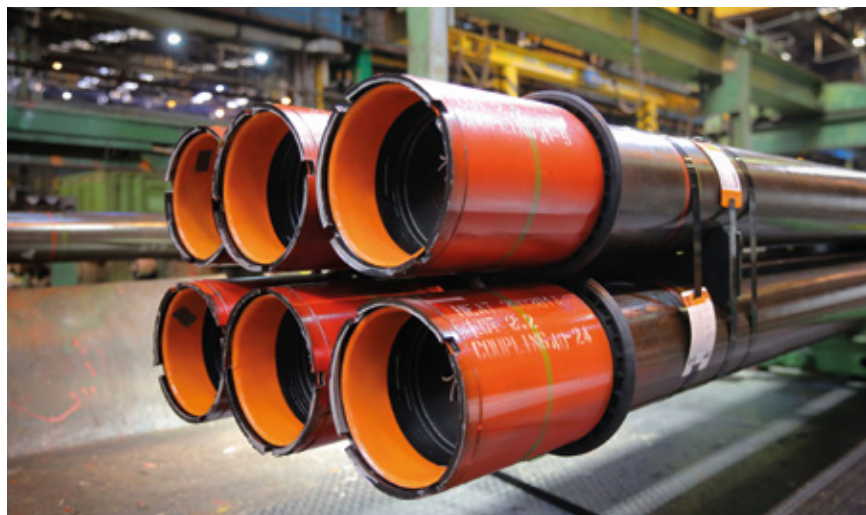
Pipes with threaded connections of latest generation | © Photo: Gazprom
