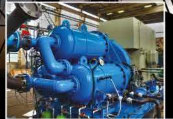
Natural gas compression equipment with helical compressors.
